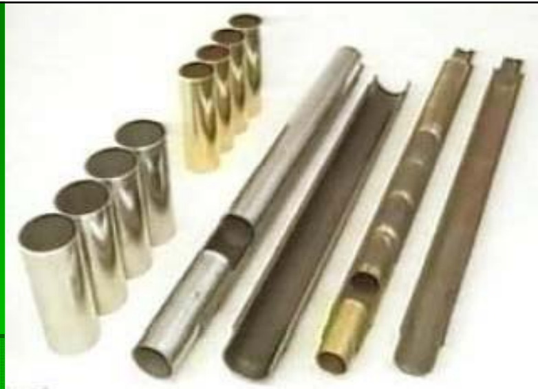
Split barrel sampler + retainer rings (Stainless steel and brass)
